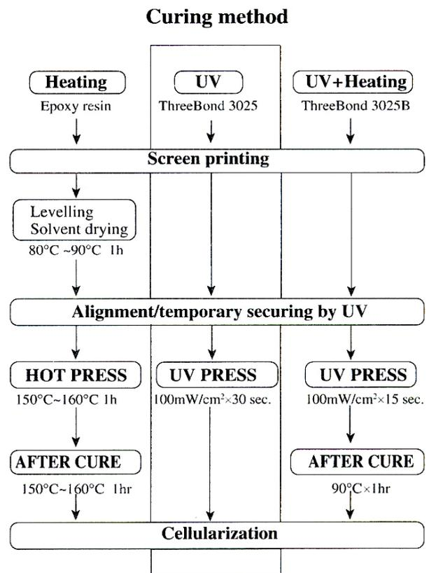
Fig. 5 Comparison of liquid crystal cell fabrication
