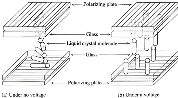
Fig. 1 Configuration of TN type liquid crystal cell
