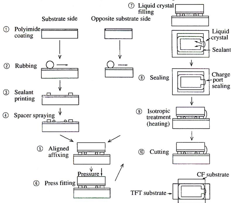
Fig. 4 Liquid crystal fabrication process
