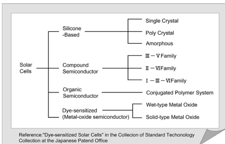
Figure 1, Classification of solar cells
