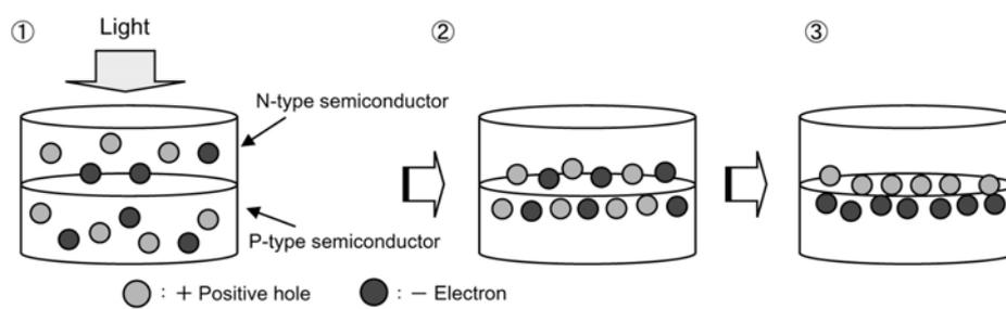
1. Pairs of electron (-) and positive hole (+) have occurred when sunshine hits semiconductor.
