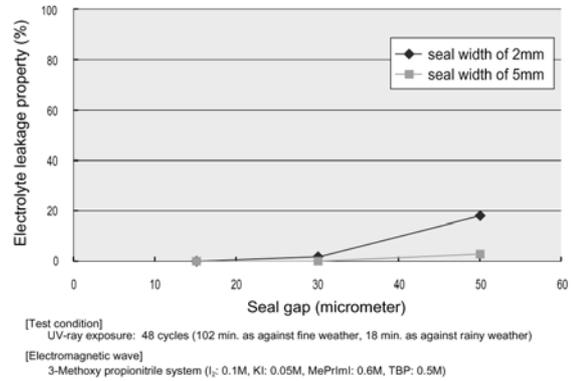
Figure 9, Relationship between seal width and seal gap
