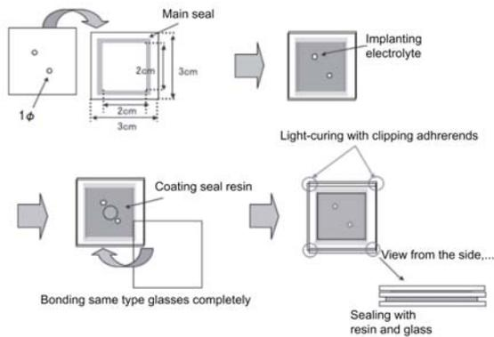
Figure 7, How to create dummy cells
