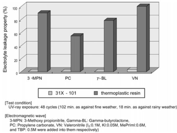
Figure 11, Comparison with thermoplastic resin on several electrolytes
