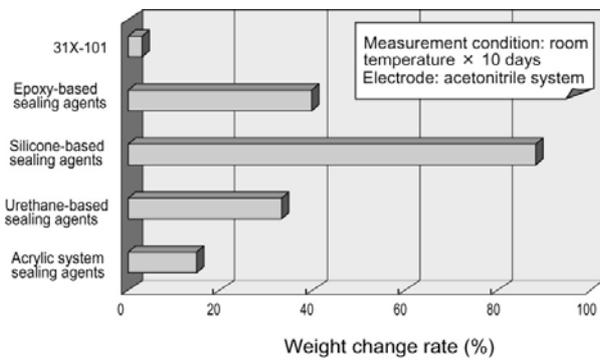
Figure 6, Comparison of electrolyte resistance property on several sealing agents
