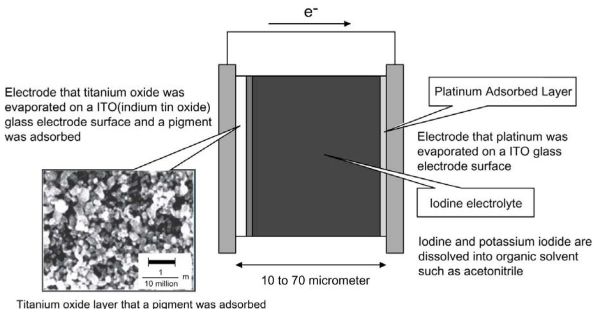
Figure 3, Overview of Dye-sensitized solar cells
