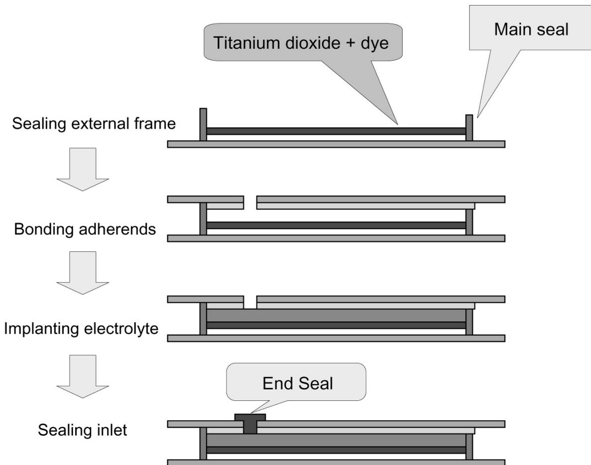
Figure 4, Conceptual diagram of DSC manufacturing process
