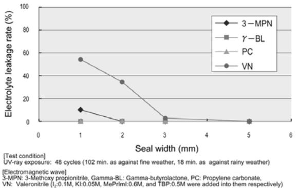
Figure 10, Sealing property on several electrolytes
