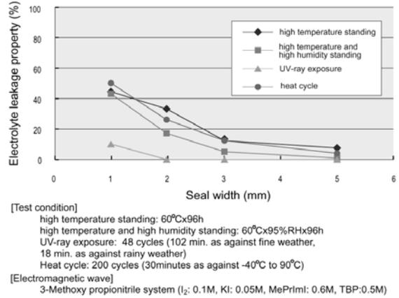
Figure 8, Sealing property on several environmental tests
