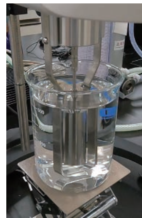
Fig. 1 B-type Viscometer (manufactured by Toki Sangyo Co., Ltd)
