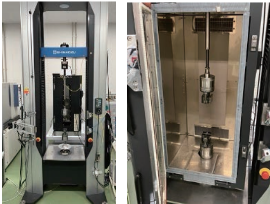
Fig. 8 Universal Tester and Measurement during Heating (tester manufactured by Shimadzu Corporation)
