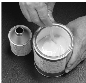
(2) Crack-detection layer coating Add curing agent and stir.
