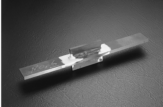
Figure 6. Welded joint test specimen
